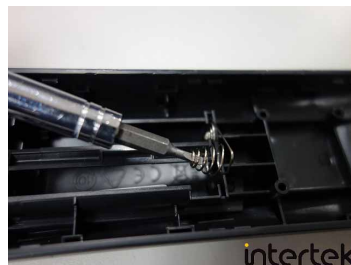
Removed the battery contact.
