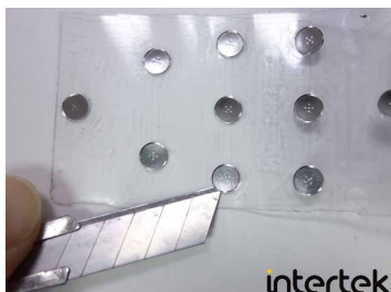
Separated the metal on the tape.
