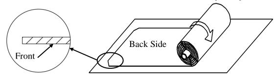
**Step 7:** Carefully and gently place the assembled frame on top of the screen material in the marked areas as shown below. Make sure to not allow the angle edge of the frame to come in direct contact with the screen material to avoid puncturing it.
