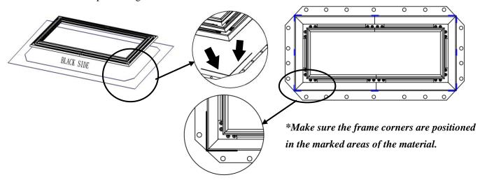
**Step 8:** Hook one end of the spring and secure inside the groove of the frame, use the *spring hook* (h) to attach the spring to the hole located on the screen material's outer edge in the following order.
