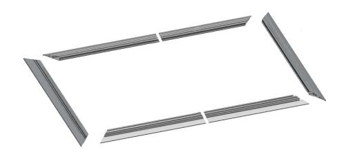
**Step 3.** Insert the *Center Joint* (*A*) connectors into one-half of the horizontal frame and secure with 4 (*M5x10mm*) screws. Once secure, connect the other half of the horizontal frame and fasten with 4 more screws.
