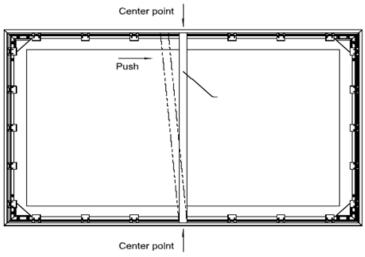
**Step 3.** Using the (M4x10) screws, screw both ends of the center support bar and make sure it is secure.
